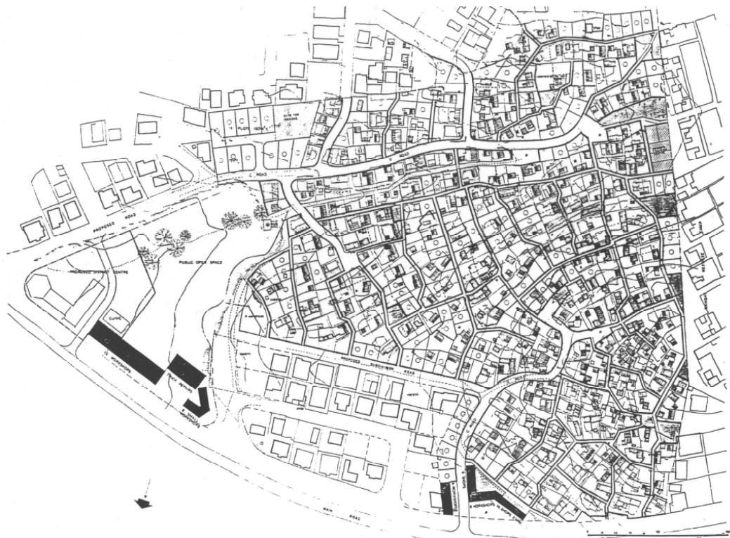
Fig 10b: Proposed layout after upgrading, retaining the traditional winding, narrow pedestrian dominated circulation pattern.
