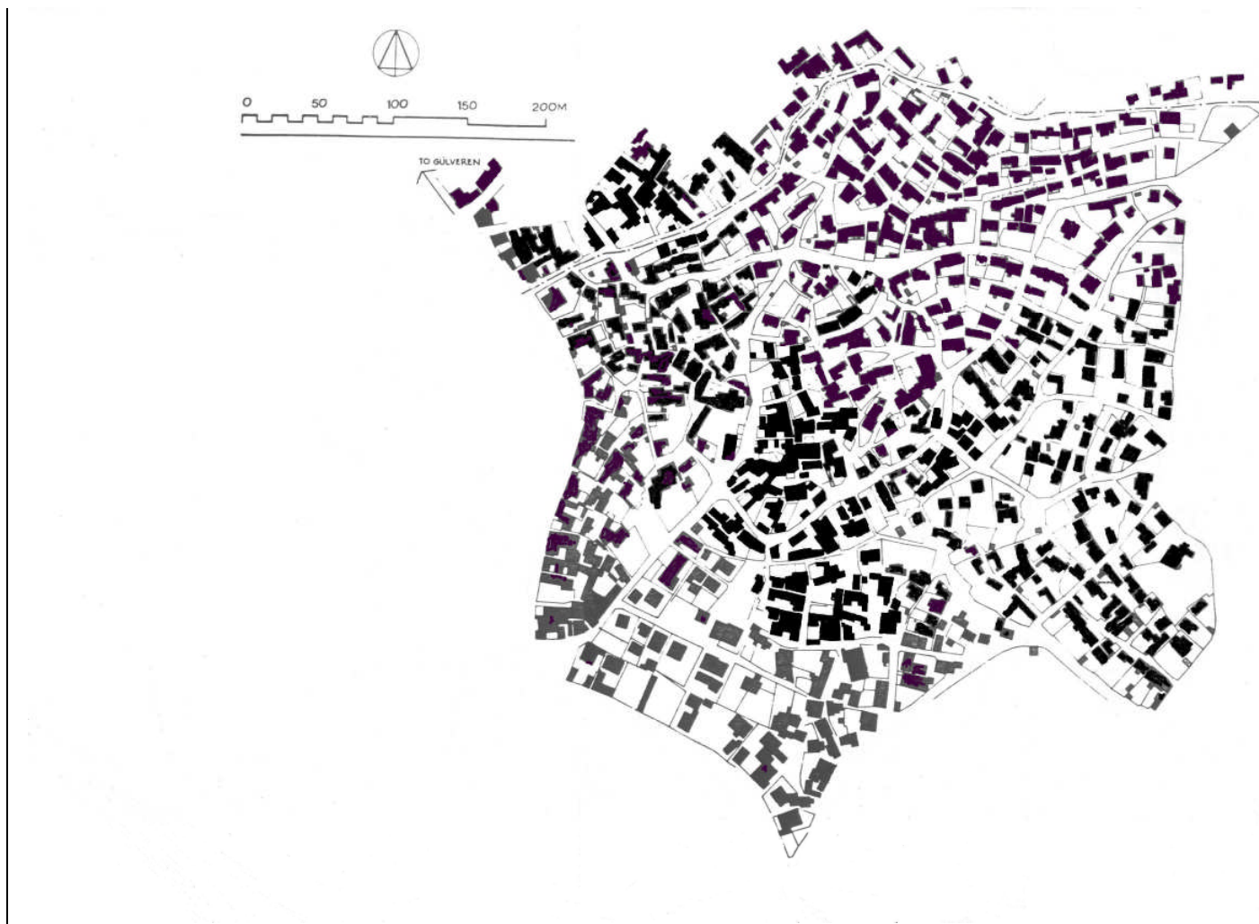
Fig 9.6: Plan of the Bahçelerüstü squatter settlement, Ankara, Turkey. Note the irregular inward-looking layout in the older area to the west, developed when the threat of official demolition was strong and the more regular, outward-looking layout in the later area to the east after the threat had receded.
